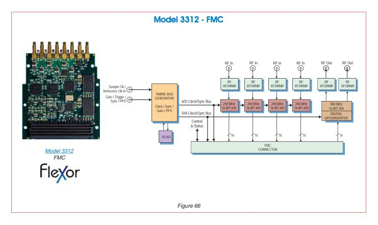
The Flexor Model <u>3312</u> is a multichannel, high-speed data converter FMC module. It is suitable for connection to HF or IF ports of a communications or radar system. It includes four 250 MHz, 16-bit A/Ds, two 800 MHz, 16-bit D/As, programmable clocking, and multiboard synchronization for support of larger high-channel-count systems.
