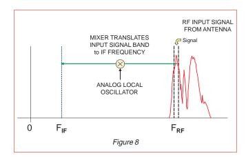
The mixer performs an analog multiplication of the two inputs and generates a difference frequency signal.
