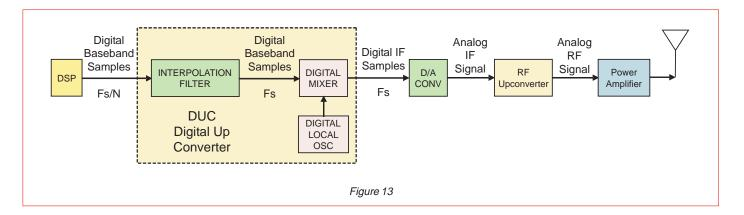
The input to the transmit side of an SDR system is a digital baseband signal, typically generated by a DSP stage as shown in Figure 13 above.
