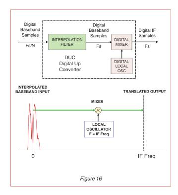
Figure 16 is a frequency domain view of the digital upconversion process.
