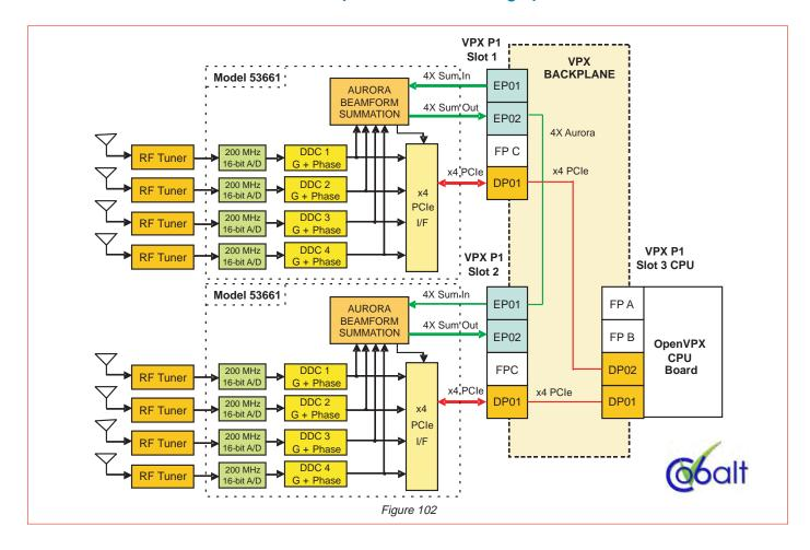
Two Model 53661 boards are installed in slots 1 and 2 of an OpenVPX backplane, along with a CPU board in slot 3. Eight dipole antennas designed for receiving 2.5 GHz signals feed RF Tuners containing low noise amplifiers, local oscillators and mixers. The RF Tuners translate the 2.5 GHz antenna frequency signal down to an IF frequency of 50 MHz.
