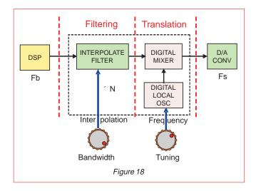
Figure 18 shows the two-step processing performed by the digital upconverter:
