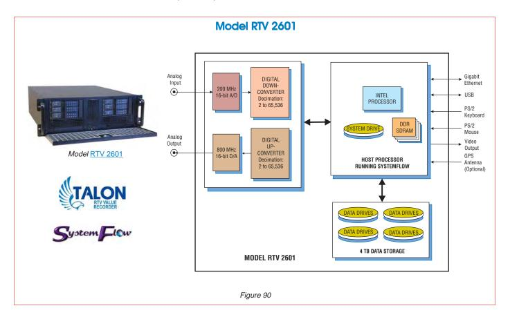
The Talon RTV 2601 is a turnkey multiband recording and playback system used for recording and reproducing signals with bandwidths up to 80 MHz. The RTV 2601 uses a 16-bit, 200 MHz A/D converter to provide real-time sustained recording rates to disk of up to 400 MB/sec. The A/D is complemented with a 16-bit 800 MHz D/A that provides the ability to reproduce signals captured in the field.
