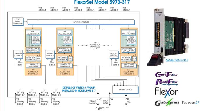
Model <u>5973-317</u> is a member of the Flexor family of high-performance 3U VPX boards based on the Xilinx Virtex-7 FPGA.
