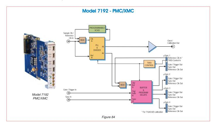
The Model 7192 High-Speed Synchronizer and Distribution Board synchronizes multiple Pentek Cobalt or Onyx modules within a system. It enables synchronous sampling and timing for a wide range of multichannel high-speed data acquisition, DSP, and software radio applications. Up to four modules can be synchronized using the 7192, with each receiving a common clock along with timing signals that can be used for synchronizing, triggering and gating functions.
