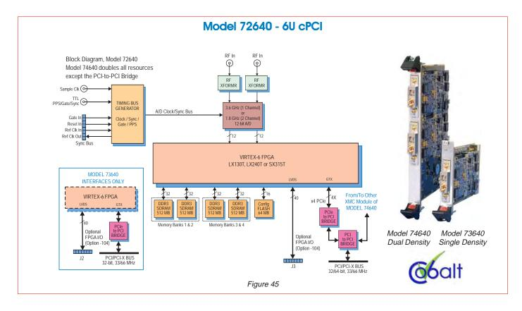
Models 72640, 73640 and 74640 are members of the Cobalt family of high-performance CompactPCI boards based on the Xilinx Virtex-6 FPGA. They consist of one or two Model 71640 XMC modules mounted on a cPCI carrier board. These models include one or two 3.6 GHz, 12-bit A/D converters and four or eight banks of memory.
