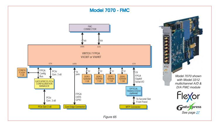
The Flexor Model <u>7070</u> is a high-performance PCIe board based on the Xilinx Virtex-7 FPGA. As a standalone processor board, it provides an ideal development and deployment platform for demanding signal processing applications.
