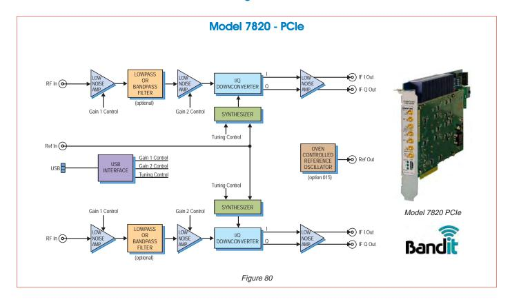
The Bandit® Model 7820 is a two-channel, high-performance, stand-alone analog RF wideband down-converter. Packaged in a small, shielded PCIe board with front-panel connectors for easy integration into RF systems, the board offers programmable gain, high dynamic range and a low noise figure.
