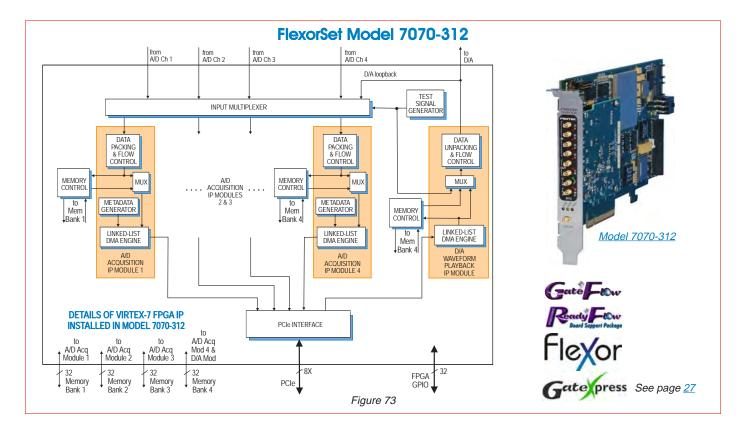
Model <u>7070-312</u> is a member of the Flexor family of high-performance PCIe boards based on the Xilinx Virtex-7 FPGA.
