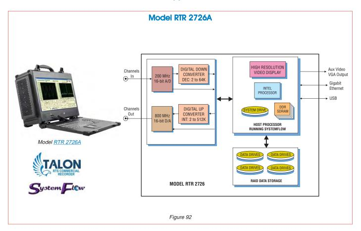
The Talon RTR 2726A is a turnkey, multiband recording and playback system that allows the user to record and reproduce high-bandwidth signals with lightweight, portable and rugged packages. This model provides aggregate recording rates of up to 3.2 GB/sec and is ideal for the user who requires both portability and solid performance in a compact recording system.
