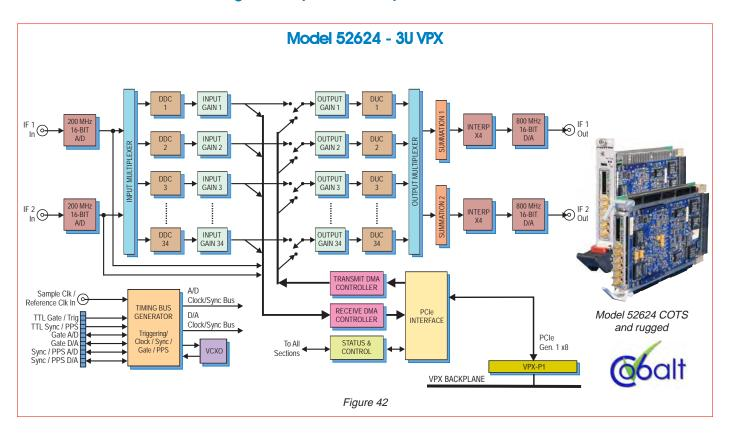
Model 52624 is a member of the Cobalt family of high-performance 3U VPX boards based on the Xilinx Virtex-6 FPGA. As an IF relay, it accepts two IF analog input channels, modifies up to 34 signals, and then delivers them to two analog IF outputs. Any signal within each IF band can be independently enabled or disabled, and changed in both frequency and amplitude as it passes through the board.
