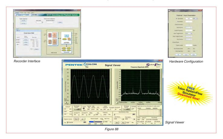
The Pentek SystemFlow Recording Software for Analog Recorders provides a rich set of function libraries and tools for controlling all Pentek analog high-speed real-time recording systems. SystemFlow software allows developers to configure and customize system interfaces and behavior.
