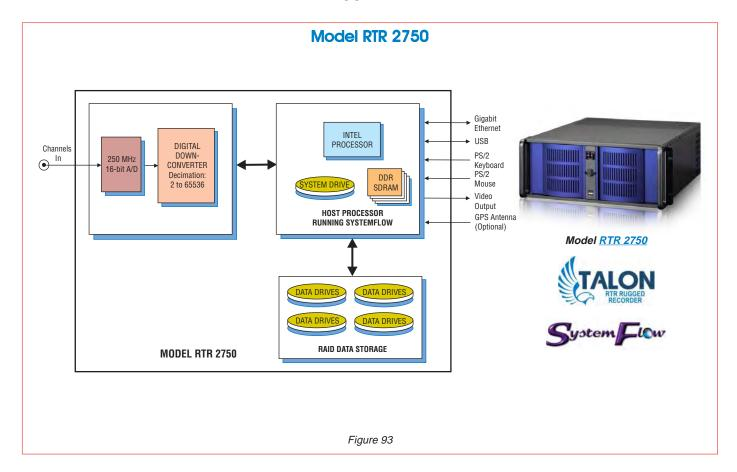
The Talon RTR 2750 is a turnkey recording system that provides phase-coherent recording of 16 independent input channels. Each input channel includes a 250 MHz 16-bit A/D and an FPGA-based digital down-converter with programmable decimations from 2 to 65536, thereby providing the ability to capture RF signals with bandwidths up to 100 MHz.
