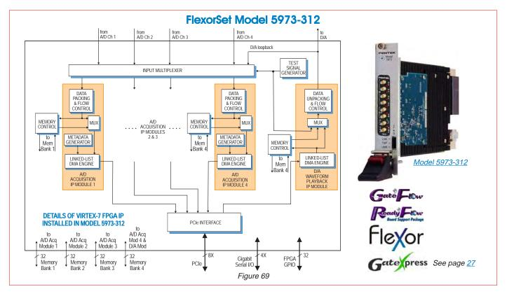
Model <u>5973-312</u> is a member of the Flexor family of high-performance 3U VPX boards based on the Xilinx Virtex-7 FPGA.
