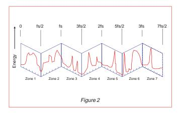
Use the vertical axis of the fan-fold paper for signal energy and plot the frequency spectrum of the signal to be sampled, as shown in Figure 2. To see the effects of sampling, collapse the transparent fan-fold paper into a stack.
