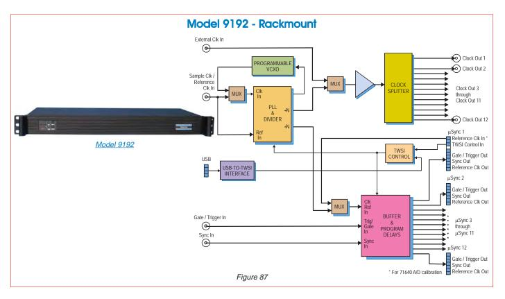
Model 9192 Rack-mount High-Speed System Synchronizer Unit synchronizes multiple Pentek Cobalt or Onyx modules within a system. It enables synchronous sampling and timing for a wide range of multichannel high-speed data acquisition, DSP, and software radio applications. Up to twelve boards can be synchronized using the 9192, each receiving a common clock along with timing signals that can be used for synchronizing, triggering and gating functions.
