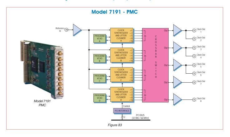
Model 7191 generates up to eight synthesized clock signals suitable for driving A/D and D/A converters in high-performance real-time data acquisition and software radio systems. The clocks offer exceptionally low phase noise and jitter to preserve the signal quality of the data converters. These clocks are synthesized from programmable VCXOs and can be phase-locked to an external reference signal.
