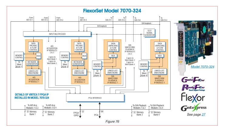
Model <u>7070-324</u> is a member of the Flexor family of high-performance PCIe boards based on the Xilinx Virtex-7 FPGA.
