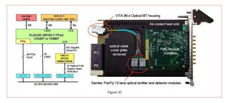
Although optical interfaces using various connectors and cable types have been deployed in embedded systems for years, most of them use front panel connections. This can be a maintenance issue and is often not permitted in conduction-cooled systems.
