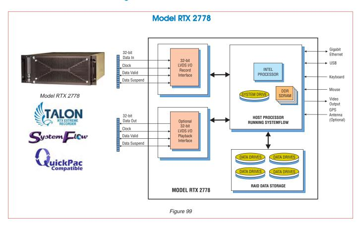
The Talon RTX 2778 is a turnkey record and playback system that is built to operate under harsh conditions. Designed to withstand high vibration and operating temperatures, the RTX 2778 is intended for military, airborne and UAV applications requiring a rugged system.
