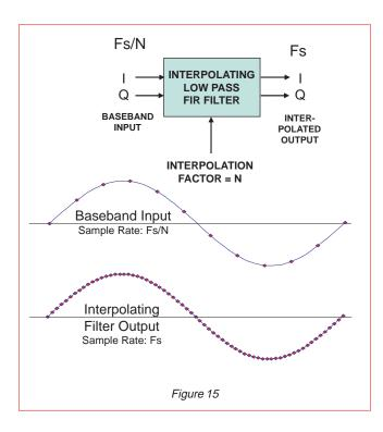
The interpolation filter must boost the baseband input sample frequency of  $f_{\rm s}$  / N up to the required mixer input and D/A output sample frequency of  $f_{\rm s}$ .
