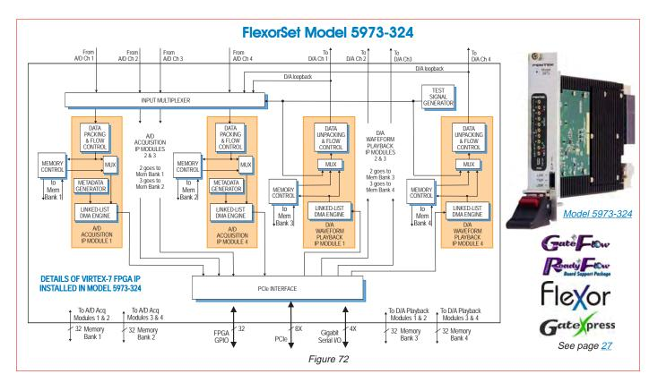
Model <u>5973-324</u> is a member of the Flexor family of high-performance 3U VPX boards based on the Xilinx Virtex-7 FPGA.
