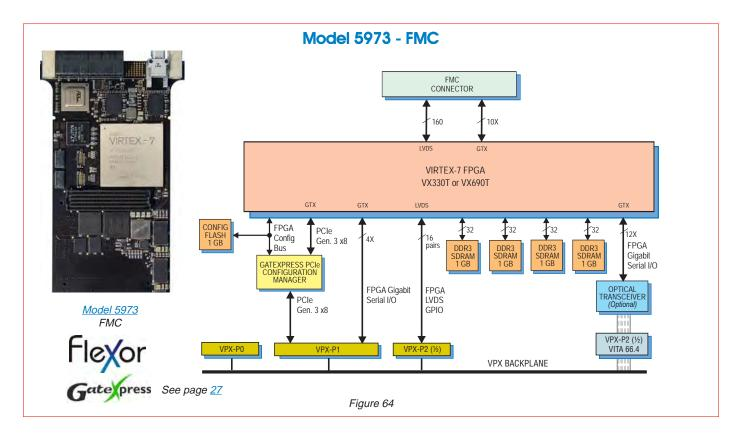
The Flexor® Model 5973 is a high-performance 3U VPX board based on the Xilinx Virtex-7 FPGA. As a stand-alone processor board, it provides an ideal development and deployment platform for demanding signal-processing applications.
