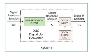
Inside the DUC shown in Figure 14, the digital mixer and local oscillator at the right translate baseband samples up to the IF frequency. The IF translation frequency is determined by the local oscillator.
