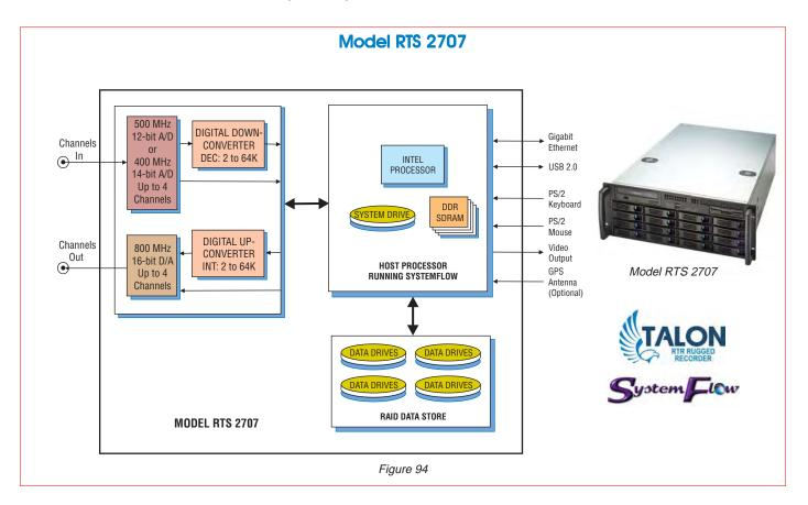
The Talon RTS 2707 is a turnkey, multiband recording and playback system for recording and reproducing high-bandwidth signals. The RTS 2707 uses 12-bit, 500 MHz A/D converters and provides agregate recording rates up to 1.6 GB/sec.
