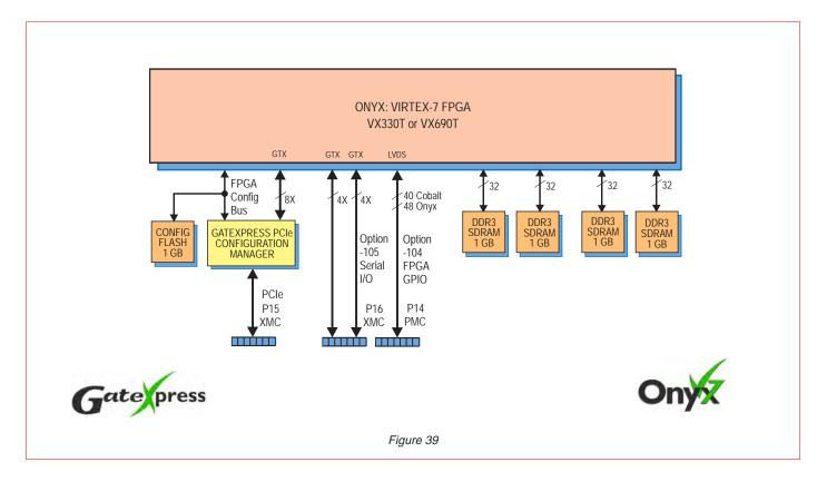
The Onyx architecture includes GateXpress<sup>®</sup>, a sophisticated FPGA-PCIe configuration manager for loading and reloading the FPGA. At power up, GateXpress immediately presents a PCIe target for the host computer to discover, effectively giving the FPGA time to load from FLASH. This is especially important for larger FPGAs where the loading times can exceed the PCIe discovery window, typically 100 msec on most PCs.
