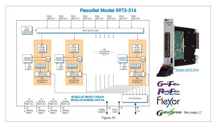
Model <u>5973-316</u> is a member of the Flexor family of high-performance 3U VPX boards based on the Xilinx Virtex-7 FPGA.
