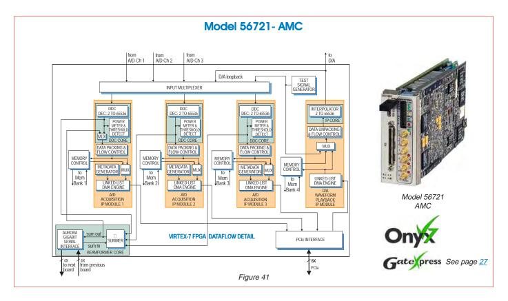
Model 56721 is a member of the Onyx family of highperformance AMC modules based on the Xilinx Virtex-7 FPGA. A multichannel, high-speed data converter based on the Model 71720 described previously, it includes factoryinstalled IP cores to enhance the performance of the 71720 and address the requirements of many applications.
