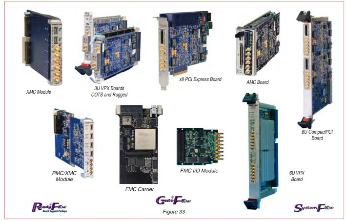
The Pentek family of board-level software radio products is the most comprehensive in the industry. All of these products are available in several formats to satisfy a wide range of requirements: PMC/XMC, PCI Express, 3U and 6U VPX, AMC, FMC, 3U and 6U CompactPCI.
