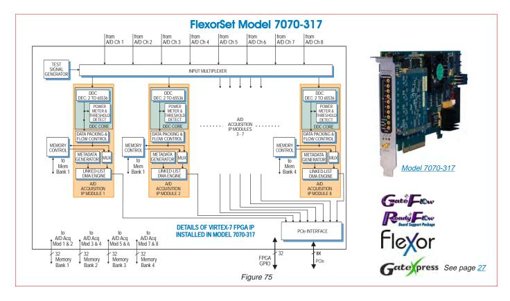
Model <u>7070-317</u> is a member of the Flexor family of high-performance PCIe boards based on the Xilinx Virtex-7 FPGA.
