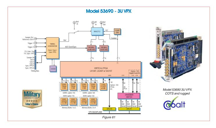
Model 53690 is a member of the Cobalt family of high-performance 3U VPX boards based on the Xilinx Virtex-6 FPGA. A 2-channel high-speed data converter, it is suitable for connection directly to the RF port of a communications or radar system. Its built-in data capture features offer an ideal turnkey solution. The Model 53690 includes an L-Band RF tuner, two 200 MHz, 16-bit A/Ds and four banks of memory. It features built-in support for PCI Express over the 3U VPX backplane.
