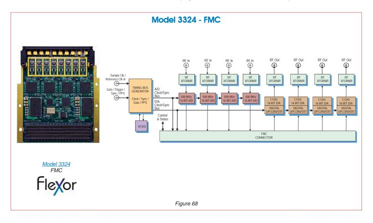
The Flexor Model 3324 is a multichannel, high-speed data converter FMC. It is suitable for connection to HF or IF ports of a communications or radar system. It includes four 500 MHz, 16-bit A/Ds, four 2 GHz, 16-bit D/As, programmable clocking, and multi-board synchronization for support of larger high-channel count systems.
