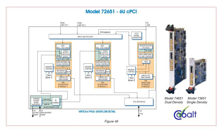
Models 72651, 73651 and 74651 are members of the Cobalt family of high-performance CompactPCI boards based on the Xilinx Virtex-6 FPGA. They consist of one or two Model 71651 XMC modules mounted on a cPCI carrier board. These models include two or four A/Ds, two or four multiband DDCs, one ot two DUCs, two or four D/As and three or six banks of memory.
