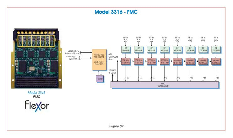
The Flexor Model <u>3316</u> is a multichannel, high-speed data converter FMC module. It is suitable for connection to HF or IF ports of a communications or radar system. It includes four 250 MHz, 16-bit A/Ds, on-board programmable clocking, and multiboard synchronization for support of larger high-channel-count systems.
