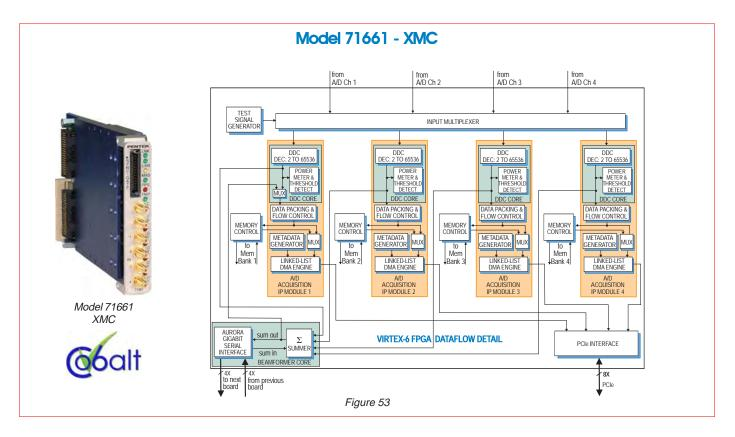
Model 71661 is a member of the Cobalt family of highperformance XMC modules based on the Xilinx Virtex-6 FPGA. A multichannel, high-speed data converter based on the Model 71660 described in the previous page, it includes factory-installed IP cores to enhance the performance of the 71620 and address the requirements of many applications.
