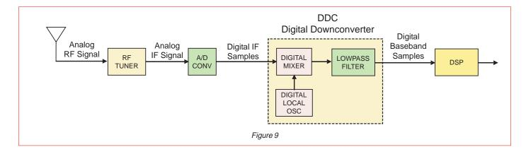
Figure 9 shows a block diagram of a software defined radio receiver. The RF tuner converts analog RF signals to analog IF frequencies, the same as the first three stages of the analog receiver.
