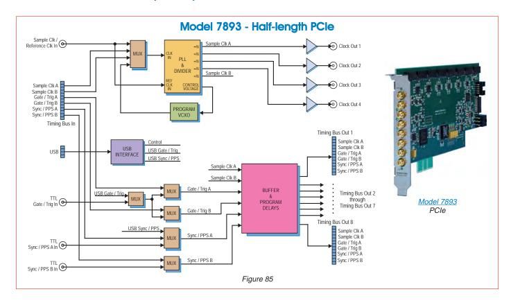
Model 7893 System Synchronizer and Distribution Board synchronizes multiple Pentek Cobalt and Onyx boards within a system. It enables synchronous sampling, playback and timing for a wide range of multichannel high-speed data acquisition, DSP and software radio applications.
