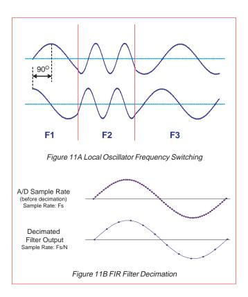
Because the local oscillator uses a digital phase accumulator, it has some very nice features. It switches between frequencies with phase continuity, so you can generate FSK signals or sweeps very precisely with no transients as shown in Figure 11A.
