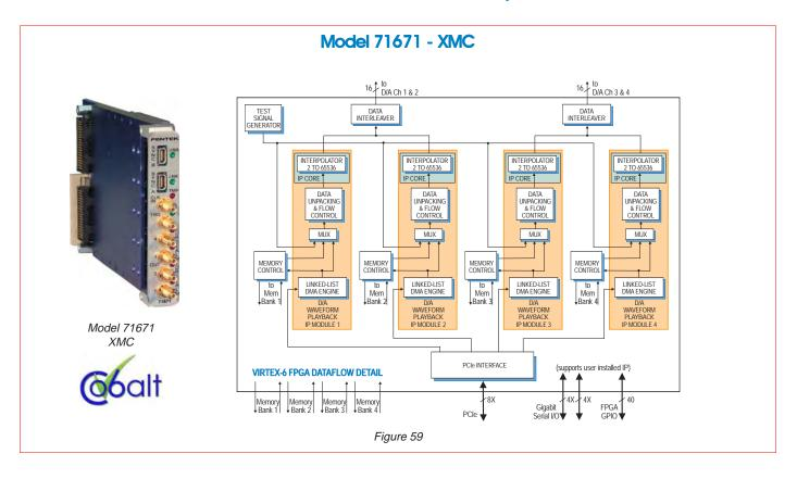
Model 71671 is a member of the Cobalt family of highperformance XMC modules based on the Xilinx Virtex-6 FPGA. A multichannel, high-speed data converter based on the Model 71670 described previously, it includes factoryinstalled IP cores to enhance the performance of the 71670 and address the requirements of many applications.
