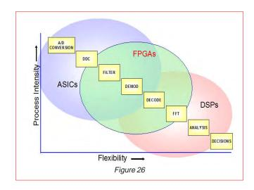
As a result, FPGAs have significantly invaded the application task space as shown by the center bubble in the task diagram above.
