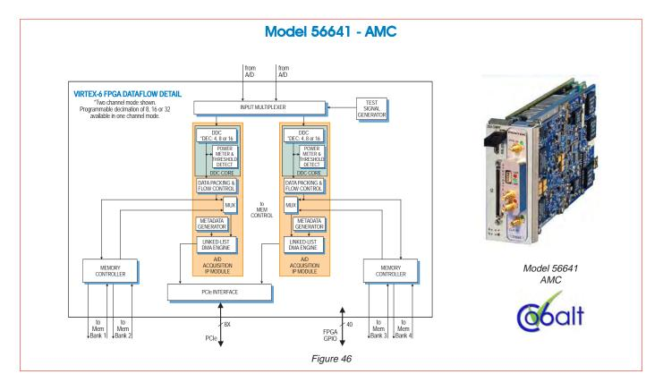
Model 56641 is a member of the Cobalt family of highperformance AMC modules based on the Xilinx Virtex-6 FPGA. A very high-speed data converter based on the Model 71640 described in the previous page, it includes additional factory-installed IP cores to enhance its performance and address the requirements of many applications.
