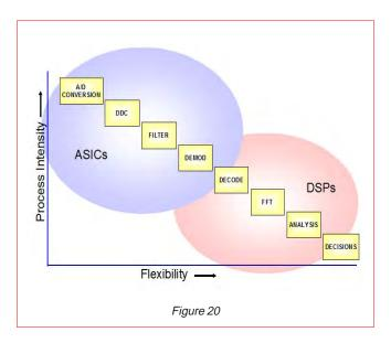
Here we've ranked some of the popular signal processing tasks associated with SDR systems on a two axis graph, with computational Processing Intensity on the vertical axis and Flexibility on the horizontal axis.
