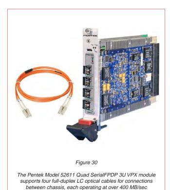
An optical cable is a waveguide for propagating light through an optical fibre. It consists of a central core clad with a dielectric material having a higher index of refraction than the core to ensure total internal reflection. Optical cables use either multi-mode or singlemode transmission.
