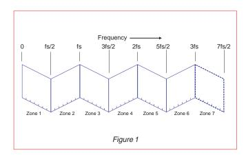
To visualize what happens in sampling, imagine that you are using transparent "fan-fold" computer paper. Use the horizontal edge of the paper as the frequency axis and scale it so that the paper folds line up with integer multiples of one-half of the sampling frequency  $f_s$ . Each sheet of paper now represent what we will call a "Nyquist Zone", as shown in Figure 1.
