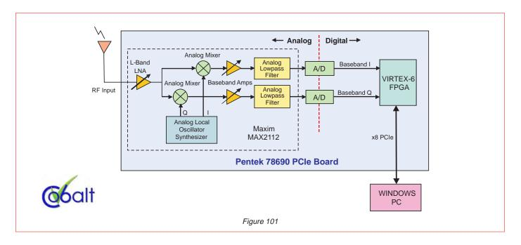
The Cobalt Model 78690 L-Band RF Tuner targets reception and processing of digitally-modulated RF signals such as satellite television and terrestrial wireless communications. The 78690 requires only an antenna and a host computer to form a complete L-band SDR development platform.
