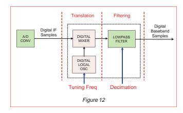
This process is called *decimation* and it means keeping one out of every N signal samples. If the decimated output sample rate is kept higher than twice the output bandwidth, no information is lost.
