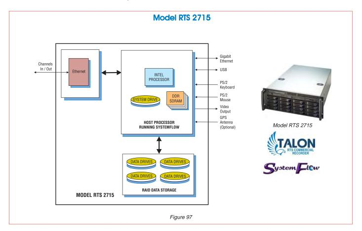
The Talon RTS 2715 is a turnkey rackmount lab recording system for storing one or two 10-gigabit Ethernet (10GbE) streams. It is ideal for capturing any type of streaming sources including live transfers from sensors or data from other computers and supports both TCP and UDP protocols. Using highly-optimized disk storage technology, the system achieves aggregate recording rates up to 1.6 GB/sec.
