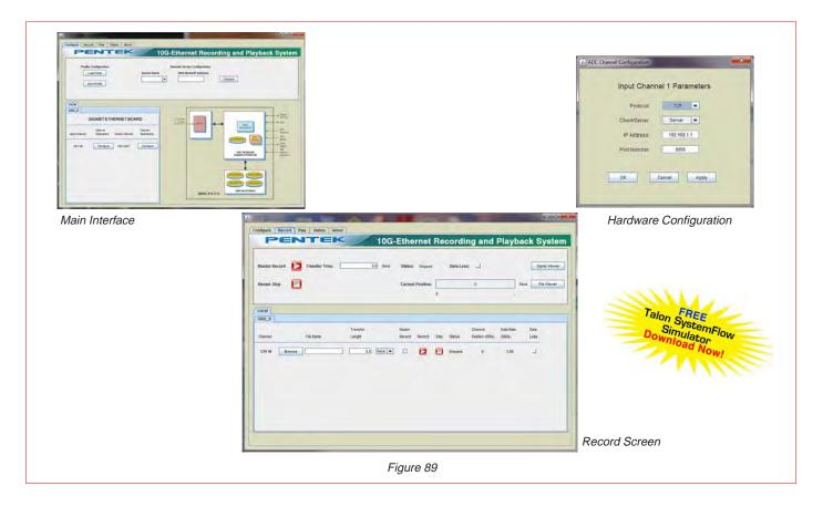
The SystemFlow Main Interface for Digital Recorders shows a block diagram of the system and provides the user with a control interface for the recording system. It includes Configuration, Record, Playback, and Status screens, each with intuitive controls and indicators. The user can easily move between screens to set configuration parameters, control and monitor a recording, and play back a recorded stream.
