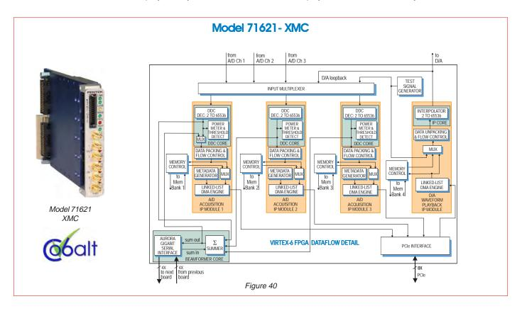
Model 71621 is a member of the Cobalt family of highperformance XMC modules based on the Xilinx Virtex-6 FPGA. A multichannel, high-speed data converter based on the Model 71620 described in the previous page, it includes factory-installed IP cores to enhance the performance of the 71620 and address the requirements of many applications.
