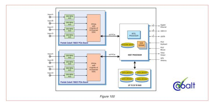
Shown above is a 64-channel recording system utilizing two Pentek Cobalt 78662 PCIe boards. The 78662 samples four input channels at up to 200 megasamples per second, thereby accommodating input signals with up to 80 MHz bandwidth.
