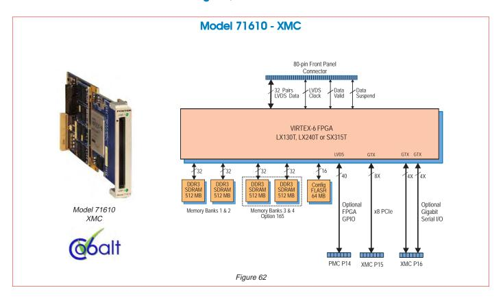
Model 71610 is a member of the Cobalt family of high-performance XMC modules based on the Xilinx Virtex-6 FPGA. This digital I/O module provides 32 LVDS differential inputs or outputs plus LVDS clock, data valid, and data flow control on a front panel 80-pin connector. Its built-in data capture and data generation feature offers an ideal turnkey solution.
