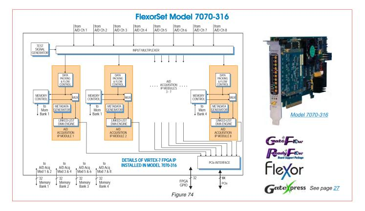
Model <u>7070-316</u> is a member of the Flexor family of high-performance PCIe boards based on the Xilinx Virtex-7 FPGA.
