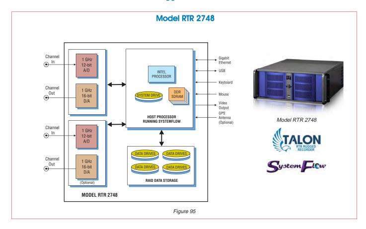
The Talon RTR 2748 is a turnkey recording and playback system that allows users to record and reproduce signals with bandwidths up to 500 MHz. The RTR 2748 can be configured as a one- or two-channel system to provide real-time aggregate recording and playback rates up to 4.0 GB/sec to an array of solid-state drives.
