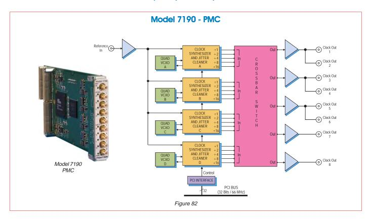
Model 7190 generates up to eight synthesized clock signals suitable for driving A/D and D/A converters in high-performance real-time data acquisition and software radio systems. The clocks offer exceptionally low phase noise and jitter to preserve the signal quality of the data converters. These clocks are synthesized from on-board quad VCXOs and can be phase-locked to an external reference signal.
