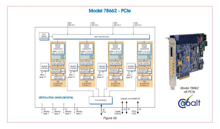
Model 78662 is a member of the Cobalt family of high-performance PCIe boards based on the Xilinx Virtex-6 FPGA. Based on the Model 71660 presented previously, this four-channel, high-speed data converter with programmable DDCs is suitable for connection to HF or IF ports of a communications or radar system.
