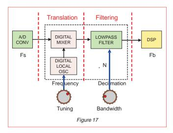
Figure 17 shows the two-step processing performed by the digital downconverter.
