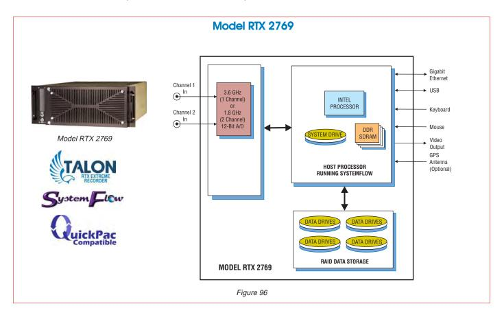
The Talon RTX 2769 is a turnkey system that is built to operate under harsh conditions. Designed to withstand high vibration and operating temperatures, the RTX 2769 is intended for military, airborne and UAV applications requiring a rugged system.
