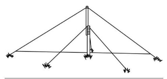
**Dimensions** The typical military half-rhombic antenna consists of a 100-foot antenna wire erected over a single 30-foot wooden mast and an 85-foot counterpoise wire placed under the antenna about one foot off the ground and attached to both ends of the antenna.
