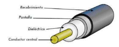
Cable coaxial detalles constructivos
