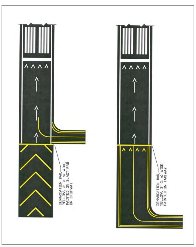
FIG 2-3-7 Markings for Blast Pads and Stopways
