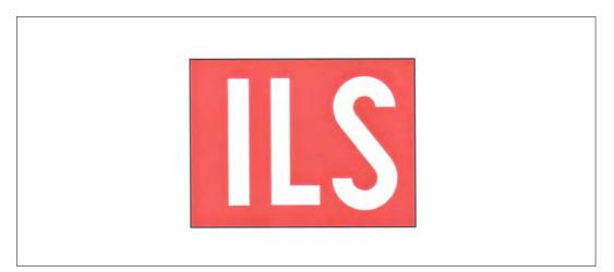
*FIG 2–3–29* Sign Prohibiting Aircraft Entry into an Area
