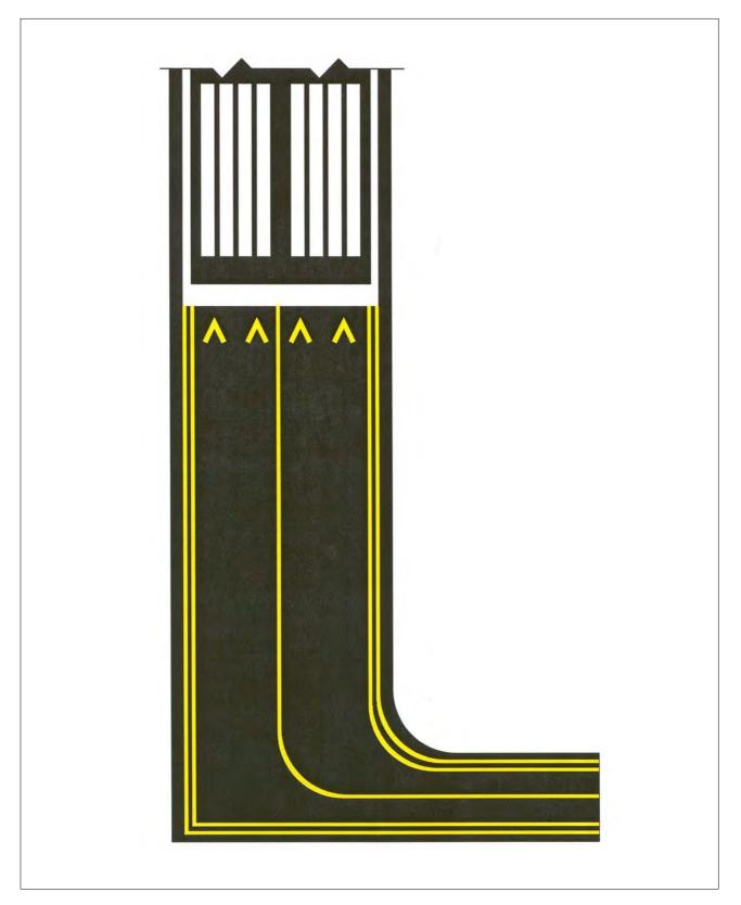
FIG 2-3-4 Displaced Threshold Markings
