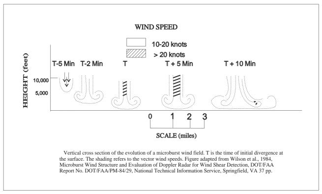
**c.** The life cycle of a microburst as it descends in a convective rain shaft is seen in FIG 7-1-14. An important consideration for pilots is the fact that the microburst intensifies for about 5 minutes after it strikes the ground.
