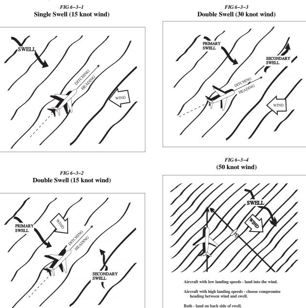
FIG 6-3-5 Wind-Swell-Ditch Heading
