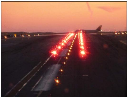
FIG 2-1-14 Taxiway Lead-On Light Configuration
