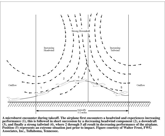
e. Microburst wind shear may create a severe hazard for aircraft within 1,000 feet of the ground, particularly during the approach to landing and landing and take-off phases. The impact of a microburst on aircraft which have the unfortunate experience of penetrating one is characterized in FIG 7–1–15. The aircraft may encounter a headwind (performance increasing) followed by a downdraft and tailwind (both performance decreasing), possibly resulting in terrain impact.
