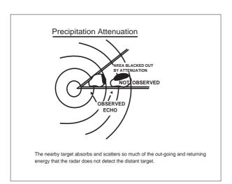
FIG 4-5-1 Limitations to Radar Service (a) The characteristics of radio waves are such that they normally travel in a continuous straight line unless they are:
