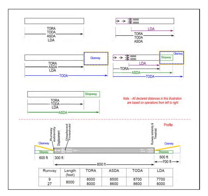
*FIG 4–3–5* Effects of a Geographical Constraint on a Runway's Declared Distances
