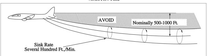
FIG 7-3-5 Vortex Movement Near Ground – No Wind
