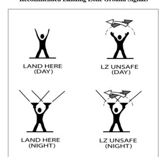
FIG 10-2-8 Recommended Landing Zone Ground Signals
