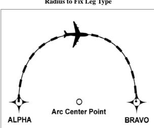
*FIG 1–2–5* Radius to Fix Leg Type
