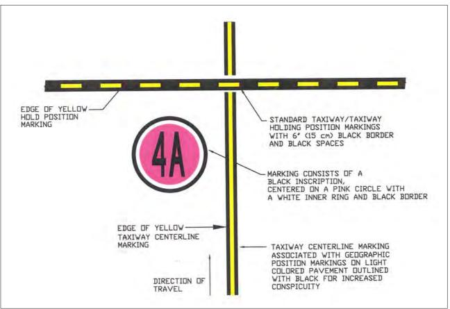
FIG 2-3-13 Runway Holding Position Markings on Taxiway
