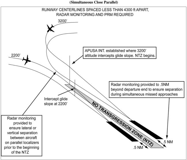
FIG 5-4-21 ILS PRM Approaches (Simultaneous Close Parallel)
