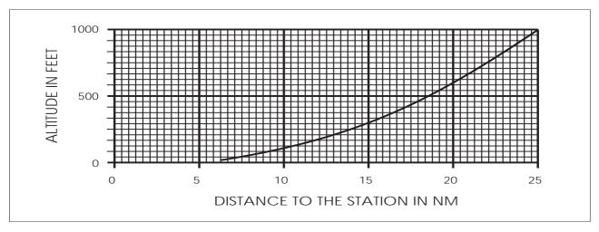
FIG 1-1-5 Service Volume Lower Edge Standard High and Low
